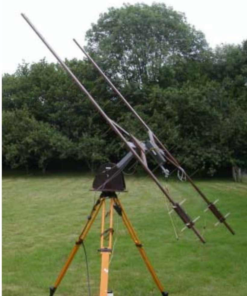
Figure 12 Antenna on a rotating stand being measured
